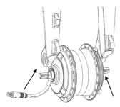
3. Mount one 2mm washer on both sides of the frame.
