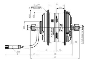
OLD: 100mm Shaft length: 142mm Motor cable length: L=250mm (optional)
